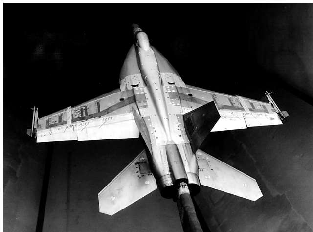
Fig. 1 F/A-18E model installed in LaRC 16-Ft TT.
